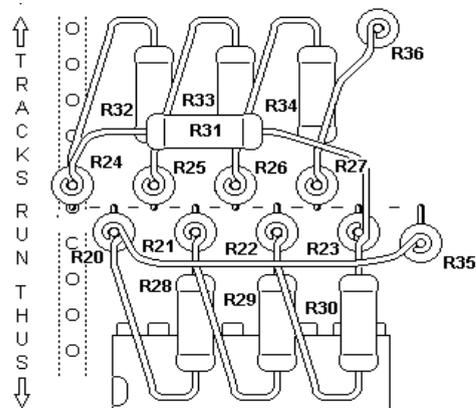
**Note** {Vertically mounted resistors R20 - R27 & R35 are in a straight line across the tracks and bent away to each side as shown diagrammatically. g16\_51f1.pcx
